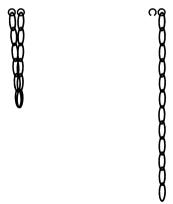
ends, and then released at one end. After the chain has finished falling, its total energy (all in the form of potential energy) is much smaller.
