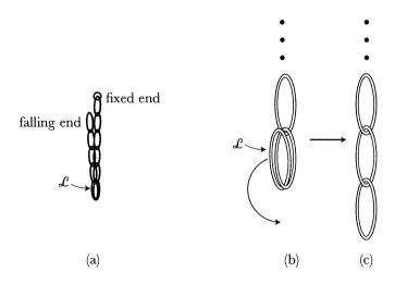
chain on the fixed end, and all that momentum will be used to yank the link around by 180°, as shown magnified in (b) and (c) of the figure. This yanking is going to pull the falling part of the chain even faster. This is basically just the opposite of what happens for the Cayley problem, where the falling chain yanks the next link off the table, resulting in the falling chain having its acceleration
