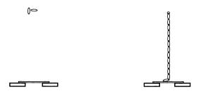
with the second, fresh, piece, and the 5 foot long chain was secured so that it hung with only the last link touching the glass. The free end was then raised to the same height as the secured end (a short distance away from it horizontally, so that the chain wouldn't become entangled in itself as it fell) and released. The result was a dramatic shattering of the glass plate.
