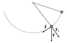
on the pendulum bob is then  $\overline{\mathbf{F}} = \mathbf{F} - \mathbf{F}_1$ , where  $\mathbf{F}$  is the conservative force from the gravitation field of the earth, while  $\mathbf{F}_1$  is the force that was introduced in our analysis, pointing along the thread. Since  $\mathbf{F}_1$  points along the thread,  $\langle \mathbf{v}, \mathbf{F}_1 \rangle = 0$ , so we still have the conservation of energy (C).
