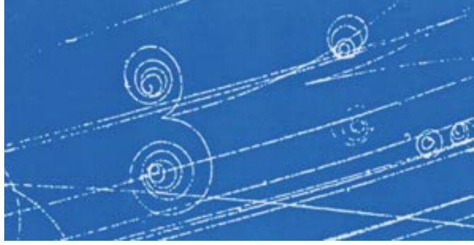
Figure 25. This bubble chamber photograph, taken at the Lawrence Berkeley Laboratory, shows a high energy \gamma ray colliding with an electron to produce an e^+e^- pair, which spiral in opposite directions. The original electron receives a huge kick and flies off to the right. At some point it emits a gamma ray which then turns into a second e^+e^- pair, this time with higher energy, visible as the V signature to the right of the picture.
